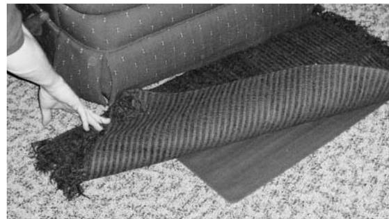
A motion sensor located under a floor mat signals when a resident moves in or out of a chair.
